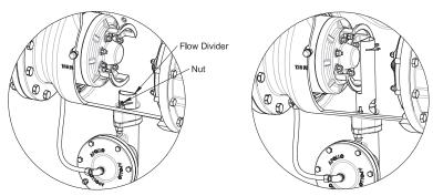
NOTE: On 10" & 12" models, the flow divider (FD) must be removed before the checks are removed. To remove the FD, remove the ¼" nut holding it in place. Then rotate the FD 90° and lift up and out of the valve body. Pay attention to which side of the body the FD is attached. The FD's tab should be oriented on the same side as the cover of the relief valve body. If the relief valve needs to be turned 180°, the FD must also be rotated 180°.
