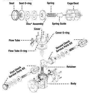
Rubber seat disc can be replaced. However, disc holder and disc retainer are permanently bonded to prevent failure.
